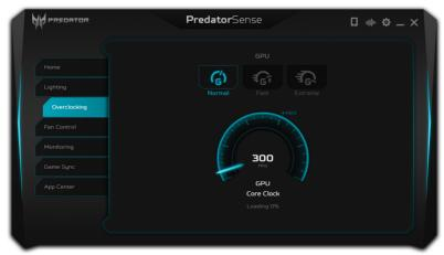
If the AC adapter is disconnected or if the battery charge is lower than 40%, overclocking options will be disabled.
